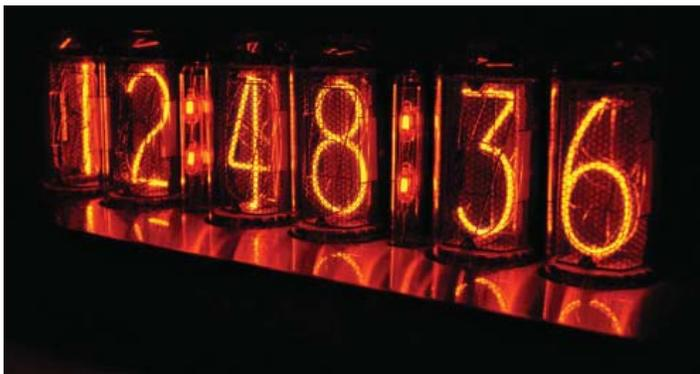
A Nixie tube (or cold cathode display, is an electronic device for displaying numerals or other information using glow discharge.
